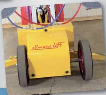
The SL 380 can be shifted sideways up to 100 mm for precision adjustment during the window installation process.
